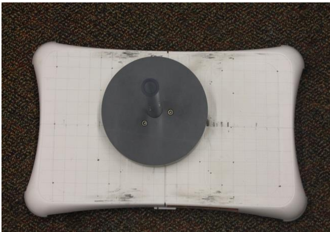
Figure 8. COP (X,Y) calibration set up
